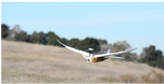
A radio-controlled robot with wings made with 40 real feathers
